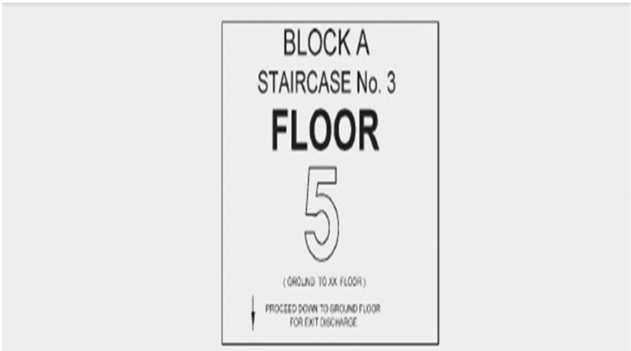
14a. Example of a Stairway Marking Sign (Floor Indication Board)
